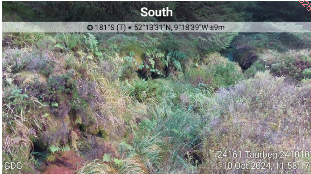
Figure 4-12: Possible peat failure scarps. Possible evidence for relict instability.
