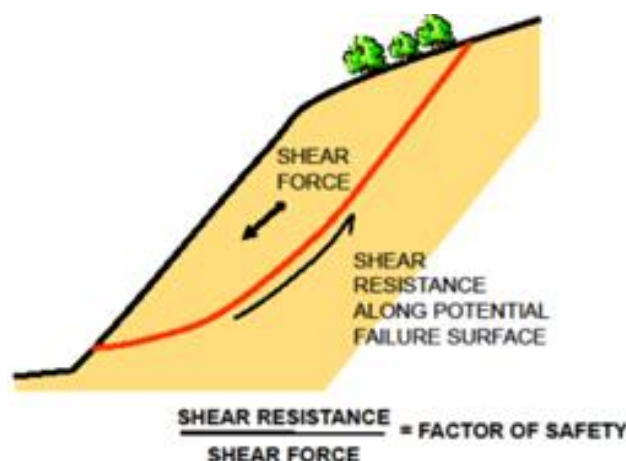
Figure 6-1: Balance of forces in a slope (Scottish Executive, 2017).
